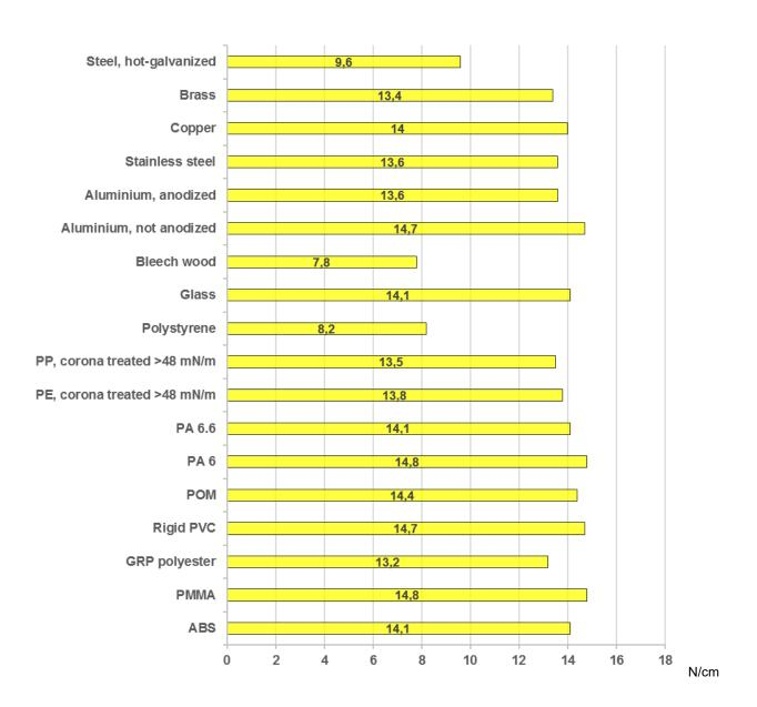
Peel strength tested according to PSTC 1. Measured with peel tester type 5966 from Instron. Load cell 10 kN, class 0,5, DIN EN ISO 7500-1 for tension and pressure, peel angle: 180°, Peel speed 300 mm/min. Printed with 21-120(T) on 50 µm polycarbonate film, measured after 24 and 72 h storage at normal climate (according DIN 50014-23/50-1).. Applied with a hand roller (according to PSTC standard: 10 pounds, rolled 5x in each direction). Adhesion area: 2,5 x 10 cm.
